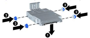
11. To place the hard drive carrier back in the chassis, align the guide screws with the slots on the drive bay, drop the carrier straight down into the drive bay (1), and press the handle on the carrier all the way down (2) so that the drive is properly seated and locked in place.
